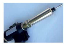
BZ 123 A with special front sleeve and nose piece for mounting of lashing rails with FERO®-BOLT blind rivets.
