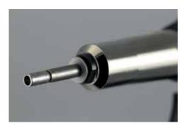
The BZ 123 A is excellently suited for working highstrength FERO®-BOLT blind rivets. To enable a guaranteed fail-safe interlocking of the mandrel, you need to use the special nose pieces shown on **>** page 203!
